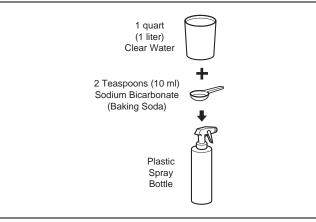
Fig. 35 Preparing Acid Neutralizing Solution
